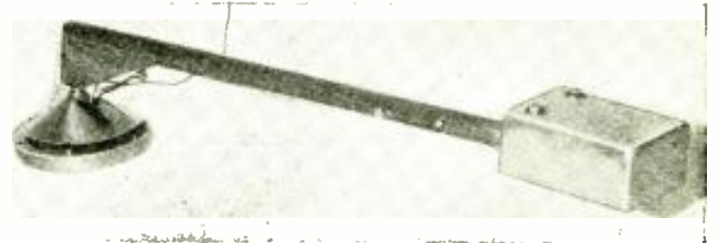
The completed pickup. Tone-arm weight is compensated by a spring.
