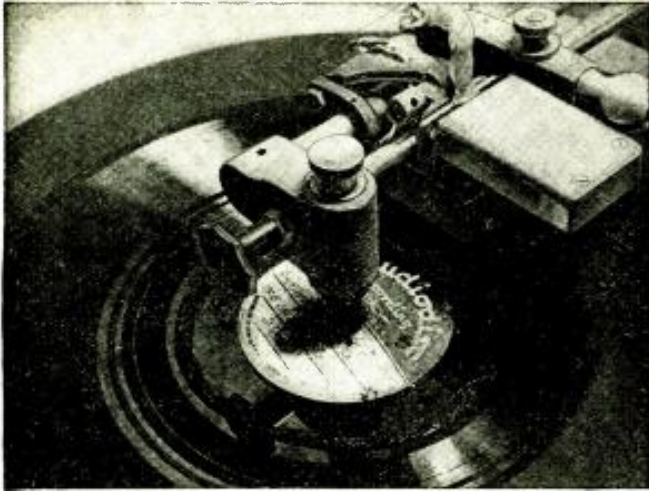
Recorder working well, chip thrown clear and moving toward center.
